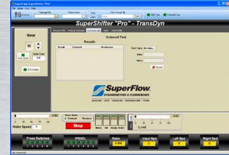
The solenoid test screen provides automated hot and cold solenoid pass fail testing. The results include pass/fail condition, which solenoid and it's resistance. Test data is stored in memory for reporting and printing. Test parameters are click-to-edit so setup is quick.
