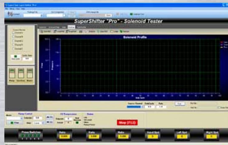
The solenoid profile screen shows the hydraulic characteristics of individual solenoids as you add power. This equates to pressure over time or response time of the solenoid.
