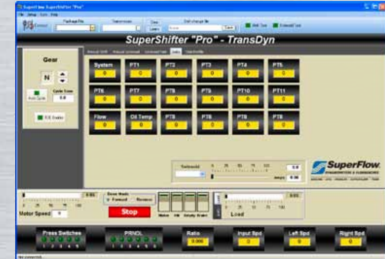
The pressure data screen displays up to 20 pressure transducers when hooked to either a valve body or transmission. Individual solenoid control from this screen allows you to see pressure change in one clutch at a time.
