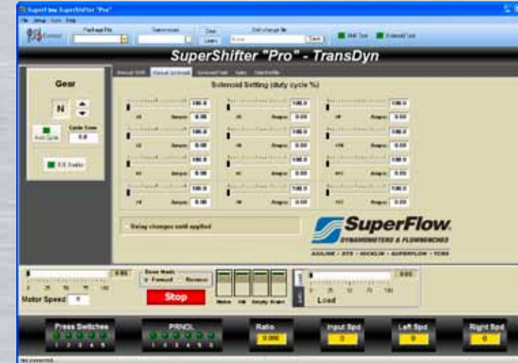
The manual solenoid control screen provides manual control or automated review of individual solenoids during shifting. The simple click-to-edit frequency ranges provide fast adjustment of solenoid response. Sliders can be pre-set and applied at once or adjusted real time individually. This screen is also useful for checking clutch slip.
